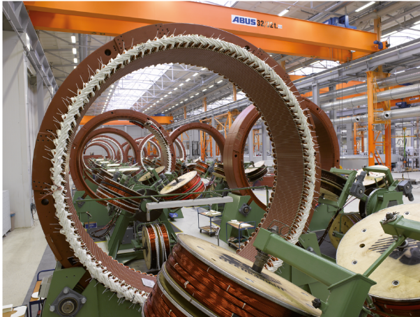
Figure 2.3.: Copper in a Generator of a big Windturbine ( Source: Enercon, www.enercon.de )
